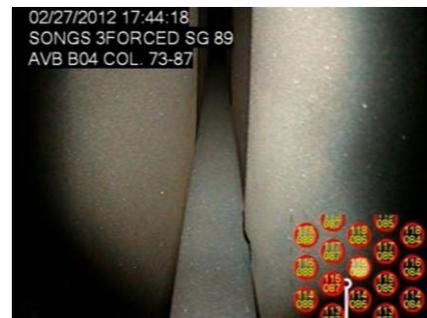
11.30.2 During normal operating conditions, or under design basis accident conditions, it is possible that fluid jets could produce damage in adjacent tubes via both droplet impact and cavitation erosion.
