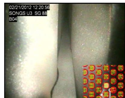
creates a wear scar that is up to x3 deeper than a scar produced by an untwisted AVB {footnote 24} and see [p76, Figure 2-18]<sup>14</sup> and other examples where the AV bar has sharply cut into the tube.
